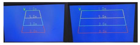
To adjust the values on the lines, go back to the main park setup menu and enter the line number menu. To modify values use the up and down keys to change the number to the required value and the Menu button to go to the next number to adjust.
