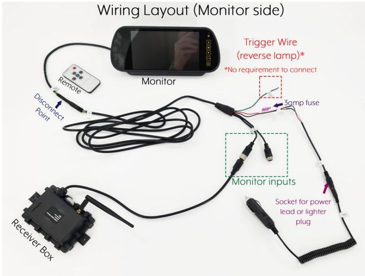
If using the lighter plug option then simply connect this to the socket (attached to the red/black wires) and insert in to your lighter socket on the vehicle.
