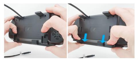
Check the monitor is firmly located against the mirror and make any small adjustments as necessary.
