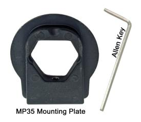
The mounting plate (MP35) adapts the hexagonal shaped windscreen button to the same shape/dimensions as a Ford/ Universal windscreen button. This then allows our Ford/Universal double ball joint swan neck bracket to fit.
