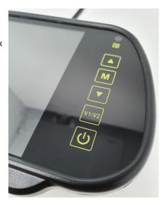
**V1/V2** - Changes between channel 1 and channel 2 of the monitor. If you only have one camera fitted, then the second channel will say "no signal"
