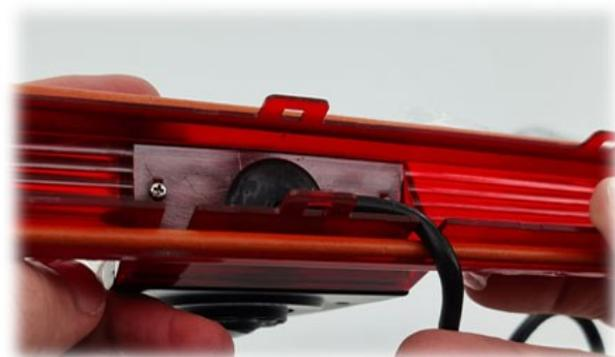
The camera cable will need to route in one of the two cutouts at the bottom
