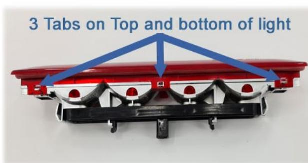
The light will have 3 tabs on the top and 3 on the bottom
