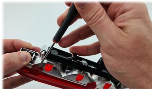
Carefully lever these up to release the light strip from the red lens
