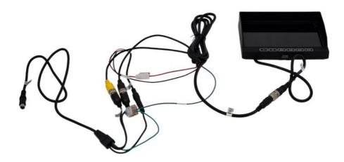
You will notice that you still use the new monitors wiring harness, but the adaptor connectors just insert in to the associated inputs of the monitor cabling. Take note of the green wire on the Adaptor 680C and the green trigger wire of the monitor. We have joined this up so that the reverse trigger feed is rescued and used to turn the monitor on automatically when in reverse.
