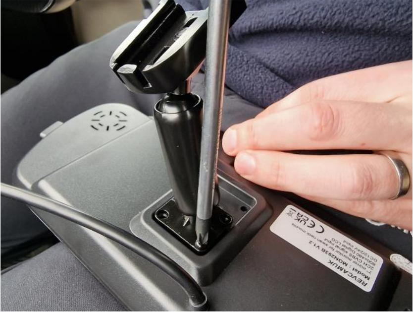
There will be 4x small screws provided with the bracket selected. Simply screw these in to 4 of the 6 screw holes located on the rear of the monitor.
