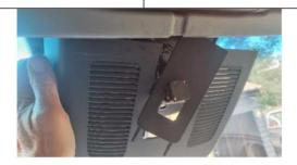
6. The final job looks like this. (Note that the mirror / screen plate does swivel but it is quite stiff and it may be easier to adjust it to the right angle before the bracket is mounted. Penetrating oil helps):
