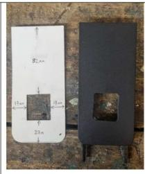
5. Put the plastic plate over the bracket, clip it back in to the plastic panel, then click the plastic panel back into place:
