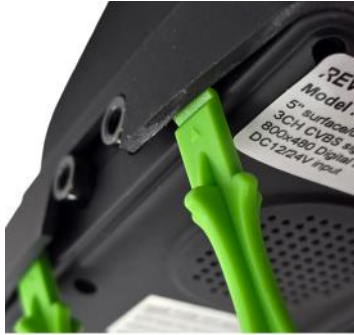
Prise the top and bottom of one side of the monitor to release the clips on sunhood
