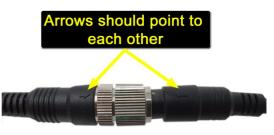
noticing the arrows that need to be lined up before pushing together.
