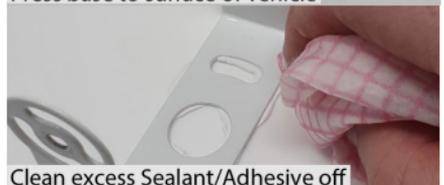
excess sealant/adhesive off before it dries to keep it looking neat and tidy. Leave to dry for recommended time. Most Sealants require 1 or 2mm thickness to work best.
