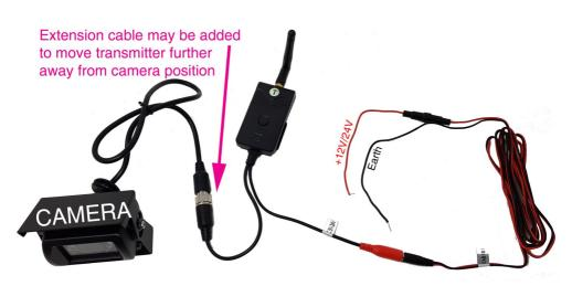
The above image shows how the transmitter side is wired up, in this picture you can see the indoor non waterproof transmitter/sender box. If you have ordered the external/waterproof boxes then the connections will be the same, the box will just look a little different.
