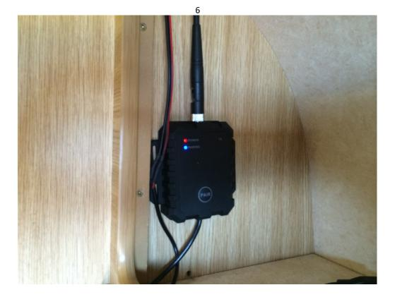
The picture above shows the sender box fitted inside a rear cupboard on the back of a caravan, the camera is mounted on the other side of this cupboard.
